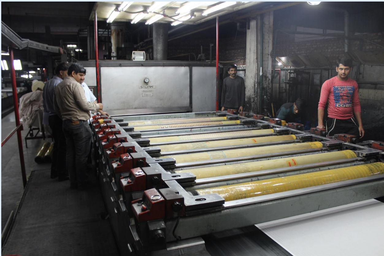
Figure-2: Rotary Printing Machine in Operation
