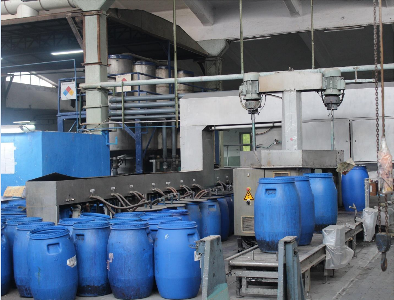
Figure-6: View of Automatic Printing Paste Dispensing System at Industry (Pakistan)
